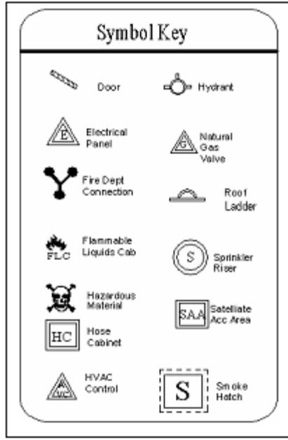
This box is used to identify the generic icons used on this drawing.
